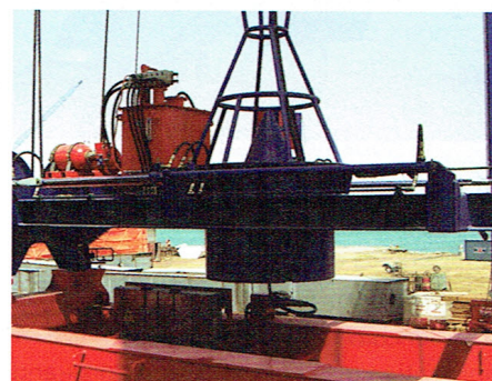
The Ruppel system allows the amplitude, and therefore the oscillation period of a container, to be reduced.
